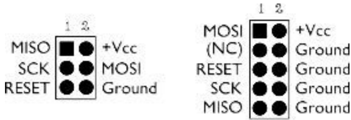
ISP Connectors: 6-pin & 10-pin
